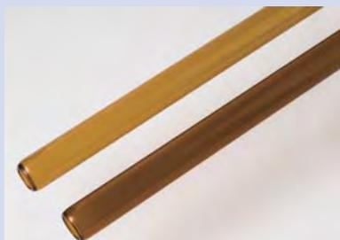
Newly developed glass tubing for pharmaceutical and medical use (below) and current model (above)
