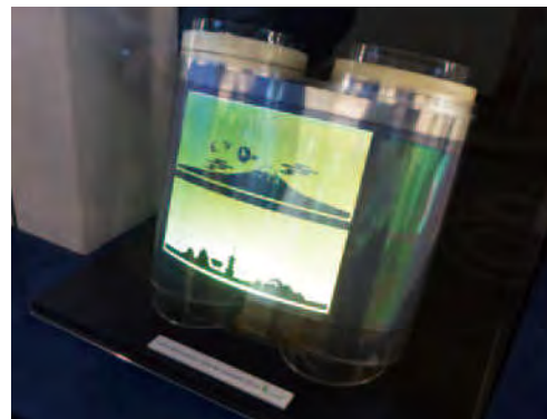
OLED lighting device made using G-Leaf™ (co-developed with Fraunhofer FEP, Germany)
