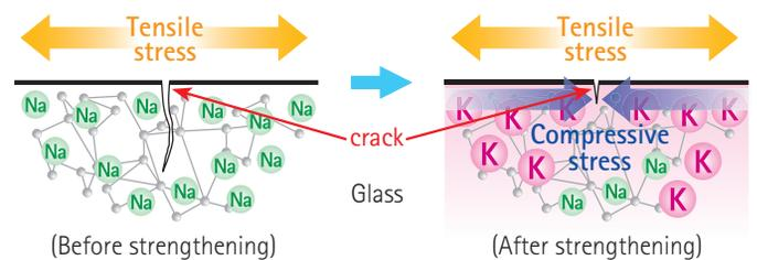
occurs in which  $\text{Na}^+$  in the surface layer of the glass is exchanged with  $\text{K}^+$ , which has a larger ion radius. This will generate high compressive stress\* in the surface layer of the glass. This process makes CX-01 so strong that it does not shatter even when smashed with a hammer.
