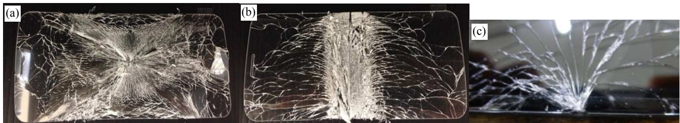
Figure 2. Crack patterns of breakage by (a) Ball Drop Test, (b) 3-Point Bending Test and (c) Typical Dropping Impact.
