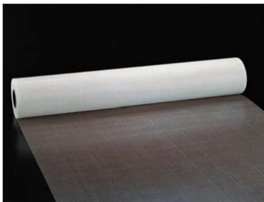
SC NET is made of glass fiber, which contains the largest content of  $ZrO_2$  commercially available.
