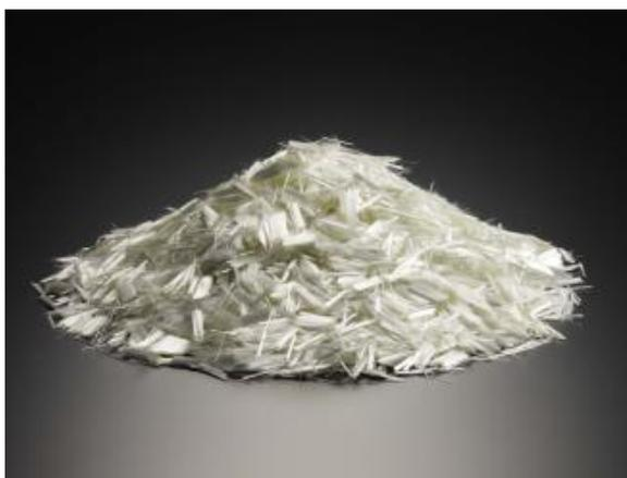
PS-750 chopped strands is water dispersible type used for water rich cementitious slurry / cement mortar. It contains some moisture and immediately disperses well in water / cementitious slurry and works as crack control at low dosage. Its filament diameter is 18 micron which is higher than S-750 chopped strands.
