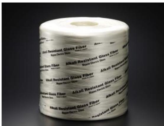
H-960 roving is multi-end assembled roving developed for excellent performance for GRC. It is especially for use with intricately shaped products in a spray-up process. The unique sizing system promotes conformity to the mold surface without bridging and creates a smooth surface.
