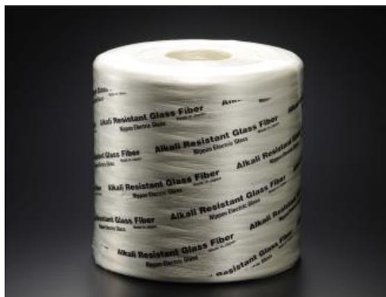
H-350Y roving is multi-end assembled roving developed for higher strength of GRC at a low dosage of the glass fiber. Its strands are a high split type with a low strand tex. It can be used for spray-up and premix processes.
